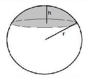
$\begin{array}{ll} \text{Spherical Cap Volume} = \frac{1}{3} * \pi * h^2 * (3r\text{-}h) \\ \text{Spherical Cap Surface Area} = 2 * \pi * r * h \\ \pi = 3.141592654 & r = \text{Sphere Radius} \\ h = \text{Cap Height} & \text{Circle Area} = \pi * r^2 \\ \text{Circle Perimeter} = 2 * \pi * r \\ \text{Sphere Volume} = \frac{4}{3} * \pi * r^3 \\ \text{Sphere Surface Area} = 4 * \pi * r^2 \\ \end{array}$
